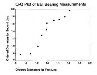
The second production line tends to have larger diameter ball bearings.
