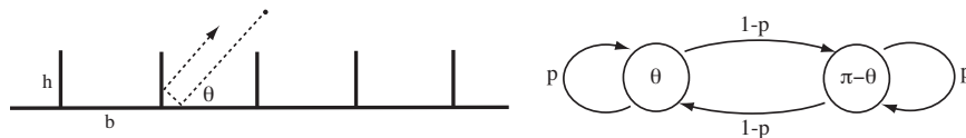
Figure 24: The scattering operator for this example is the transition matrix of an ordinary Markov chain with two states, \{\theta, \pi - \theta\} , where the initial angle satisfies 0 < \theta < \pi . The transition probabilities are given by the diagram on the right. By writing 2h/(b \tan \theta) = k + s , where k is an integer and 0 \leq s < 1 , a simple calculation shows that p = s if k is odd and p = 1 - s if k is even.
