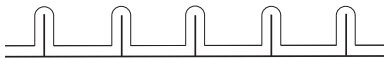
Figure 26: The hair-comb microgeometry of figure 24 does not satisfy the ergodicity condition for the validity of Knudsen’s cosine law. For this geometry the probing particle is necessarily point-like (zero radius). But the micro-geometry becomes ergodic if the probing circular molecule has non-zero radius. In this case, the same hair-comb geometry is seen by the molecular center of mass as the thickened contour in the above figure. The tip of the semicircular cap is now a point of maximal height of non-zero curvature. The existence of such a point is sufficient for the cosine law to hold.
