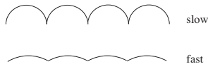
Figure 7: The top geometry, with bigger curvature, produces slower diffusion than the one at the bottom.
